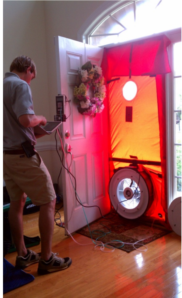
Figure 29. 'Blower Door' diagnostics test underway
